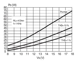
Figure 5. Output power vs. supply voltage.
