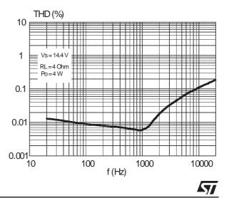
Figure 9. Distortion vs. frequency.
