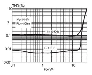
Figure 7. Distortion vs. output power
