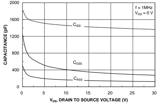
Figure 8. Capacitance Characteristics
