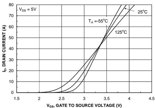
Figure 5. Transfer Characteristics
